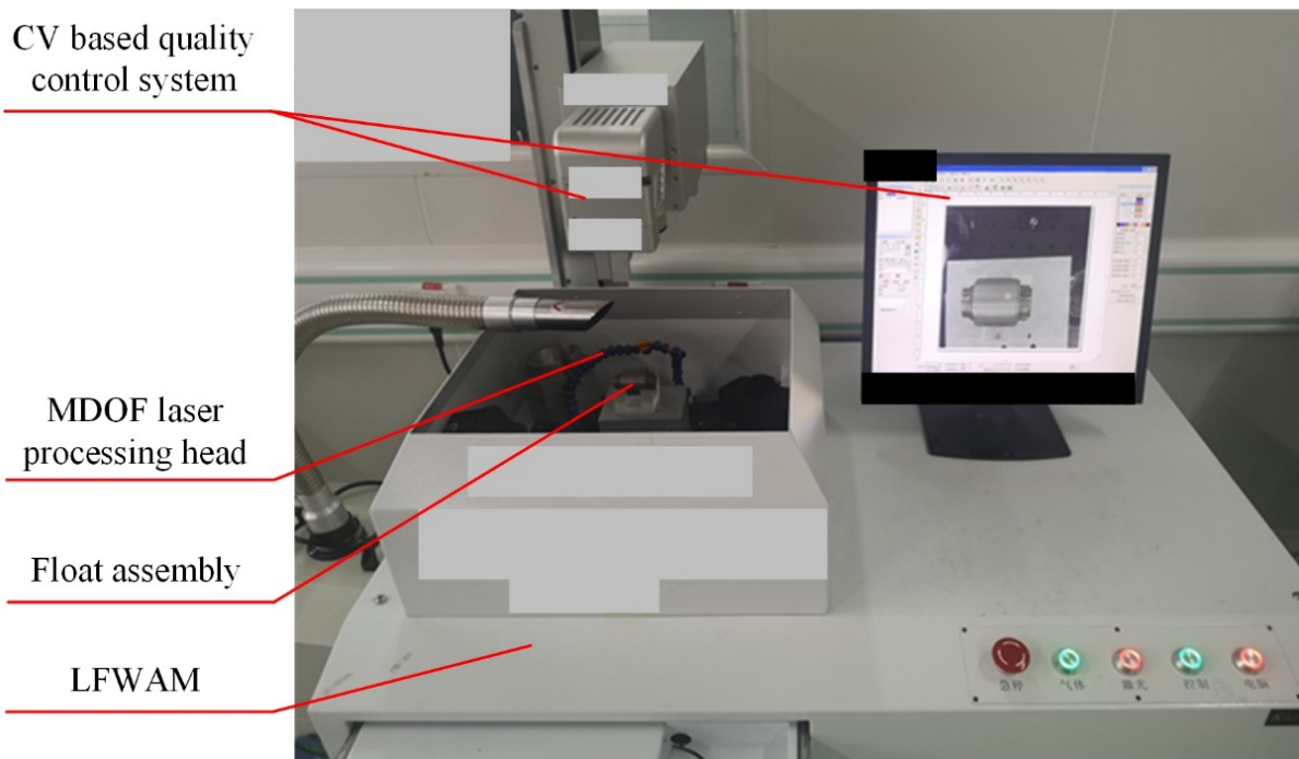
Figure 8. The developed LFWAM for the mass removal of float assembly in PIGA.
