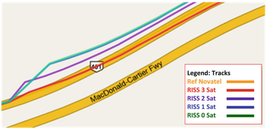
Fig. 10.22 A zoomed view of the performance of a tightly coupled 3D RISS during GPS outage #3
