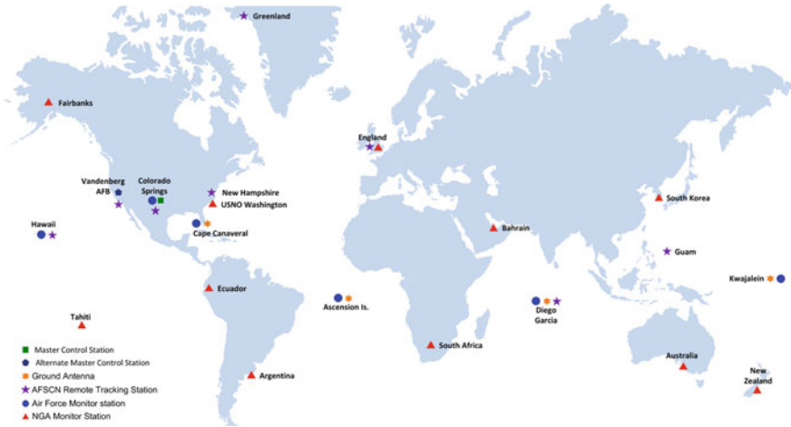
Fig. 3.6 Distribution and location of various elements of the GPS control segment
